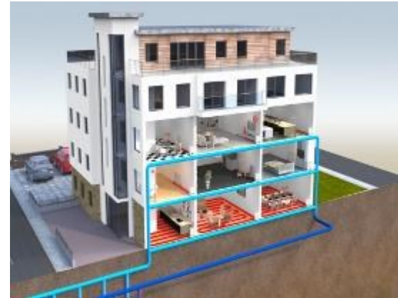
Apartment Development with a DV-A Communal ground array
